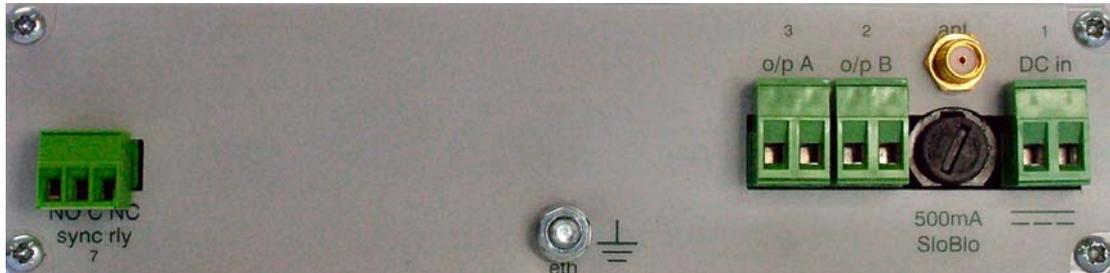
Fig 2 : TCG 1000P Rear Panel with 2-pin
