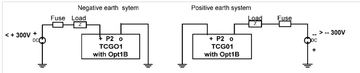
Fig 4 : High Voltage MOSFET Output Switch Option: Suggested wiring arrangements
